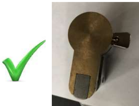
Figure 3. Adjusted lock with tab at 90 degrees
