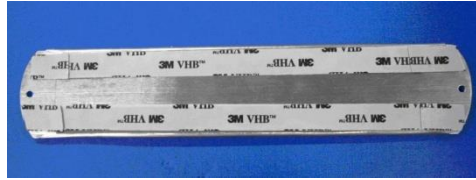
Figure 8.6 – Double-sided acrylic foam tape applied on the back of the aluminium holder
