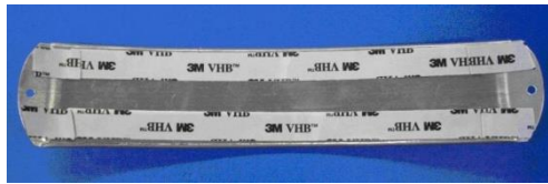
Figure 8.9 – Double-side acrylic foam tape applied on the back of the curved character holder
