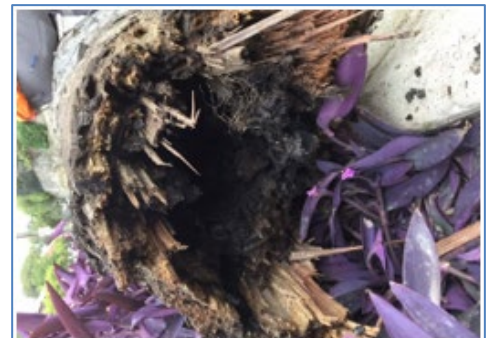
Figure 1: Internal pole decay
