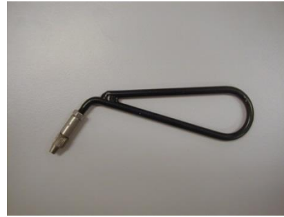
0.4mm Pirelli Insulation Screen Scoring Tool (stockcode 178198 or from Blackwoods Part No 0536 6992)
