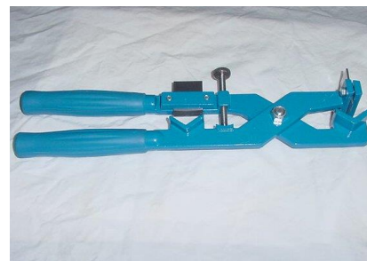
XLPE Insulation Splitting Tool (from NKT Australia Part No RKM 1055(4550.143.0)) used where there is insufficient room between cable cores to rotate the XLPE Insulation Stripping Tool
