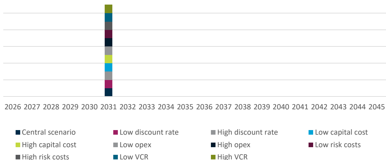
Figure 5.3 – Option 1's distribution of optimal project commissioning years under each sensitivity
