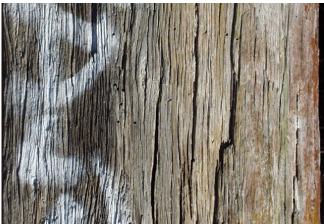
Figure 34 – Typical Glyptotermes Flight Holes Above Groundline
