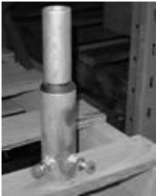
For steel standards (with clamping bolts) Drawing 125149 & 240795
