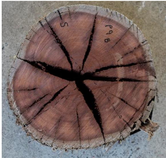
Figure 46 – Example of a pole with heart collapse, checking and splitting
