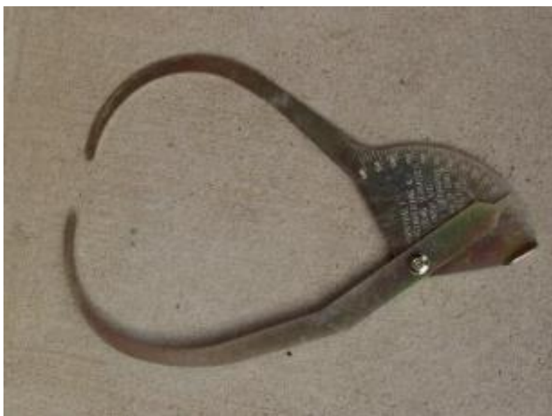
Figure 41 – Outside callipers suitable for measuring the reduced diameter
