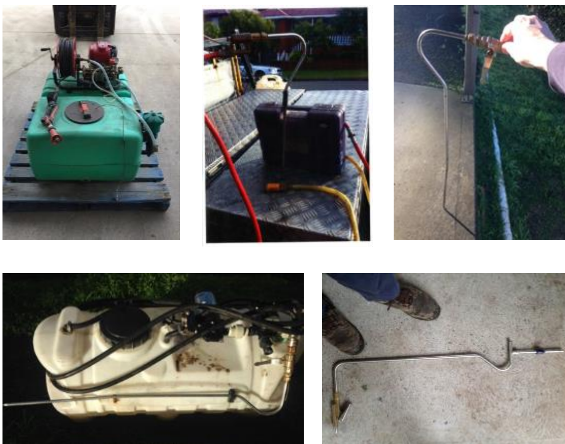
Figure 52 – Injection Equipment for Inground Barrier and Internal Pole Nest Treatment
