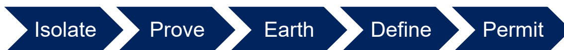
Figure 49 - Illustration of the steps required to allow work on or near high voltage mains and apparatus
