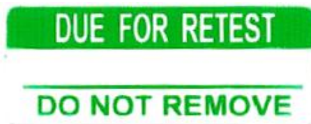
Figure 25 – An example of a test sticker for HV insulated tools
