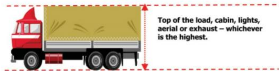
Figure 29 – An illustration of the maximum overall height of a vehicle (Image courtesy of SafeWork NSW)
