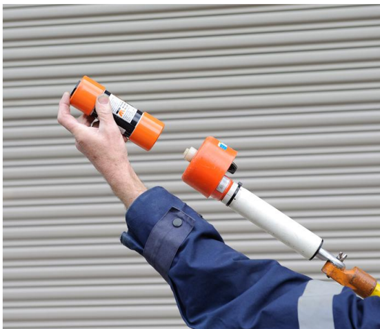
Figure 56 - Checking HV detector
