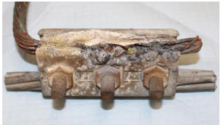
PG Clamp with copper side melting
