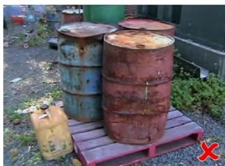
Drums in poor condition, not banded, unlabelled or uncovered can leak and contaminate land or waterways
