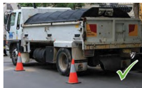
Cover loads to prevent pollution
